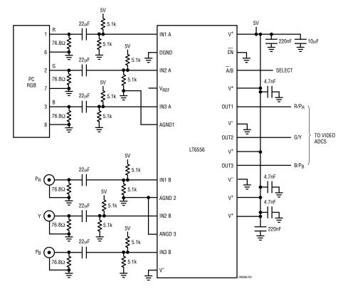
Figure 1. LT6556 Provides Input Video Selector and ADC Driver for Multimedia Display System
