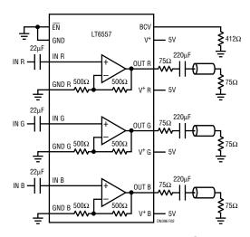
Figure 2. LT6557 Provides Low Part Count UXGA-Resolution Cable Driver on 5V Supply
